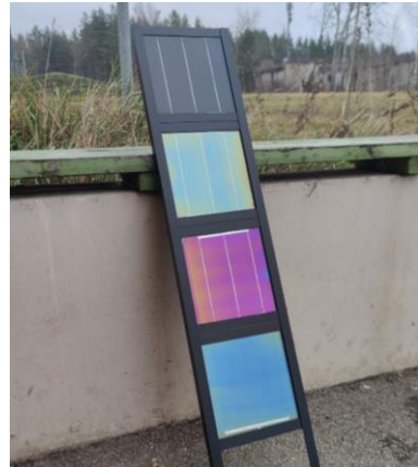
Figure 44. Upscaled 20x20 cm size mini panels with multilayered 1D photonic structures (from the top): black (REF), greenish, purple, light blue (textured glass, painted busbars – a seamless solution).
