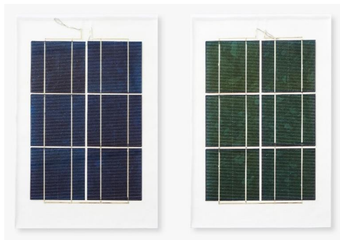
Figure 19. Glass/glass solar panels made using 6 green (185 nm ITO) and blue (0 nm ITO, reference) sequentially connected cells.
