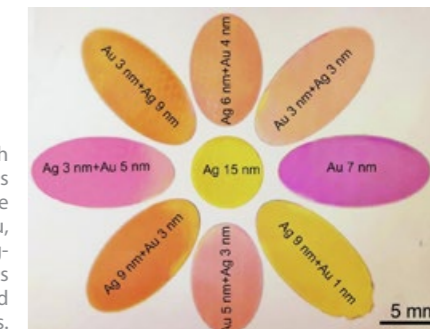
Fig. 15. Photograph of nano-particles on glass substrate obtained from Au, Ag, Au-Ag, and Ag-Au films of various thicknesses and ratios.
