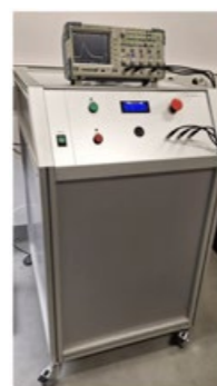
Fig. 5. 12-stage Marx pulse generator.
