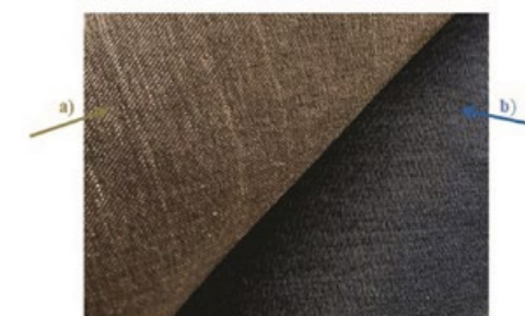
Fig. 2. PEDOT:PSS coated fabric: a) initial, b) with PEDOT:PSS coating.
