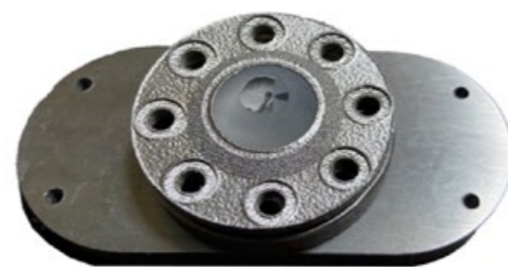
Fig. 13. Image of the nozzle with two different gas supply systems assembled into 3D metal printed support.
