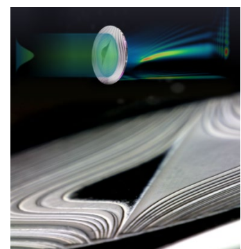
Fig. 6. Photo (main body) of Airy lens for THz structured light generation. Inset – schematic illustration of the lens performance.
