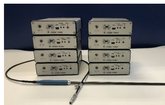
Fig. 8. B-Scalar magnetic field measurement modules with semi-flexible probe. The project was project supported by MITA (Project Nr. 01.2.2-MITA-K-702-06-0012).
