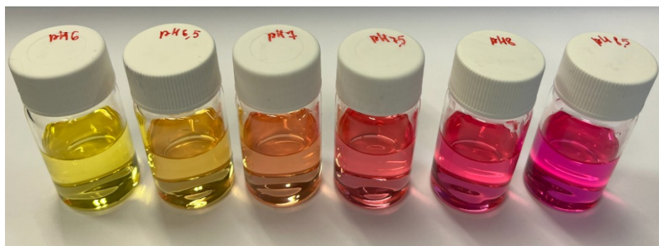
Figure 20. Visual representation of the colour variation in phenol red-containing cell culture medium corresponding to different pH levels.
