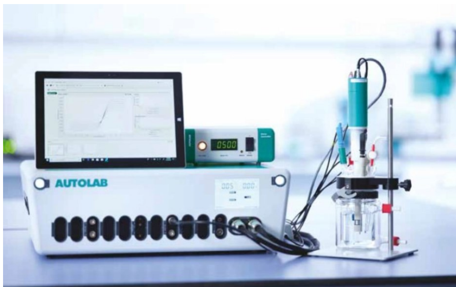
Figure 9. Representation of the potentiostat of Methrom, Autolab PGSTAT302N, used in our research. Image taken from Labx.com 209
