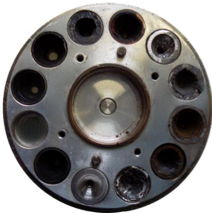
Figure 1. Negative Cs-sputtering Ion source target
