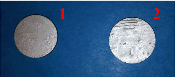
Experimental dielectric samples with permittivity of \sim 17 (1) and \sim 33 (2) for measurement in the radio frequency range.
