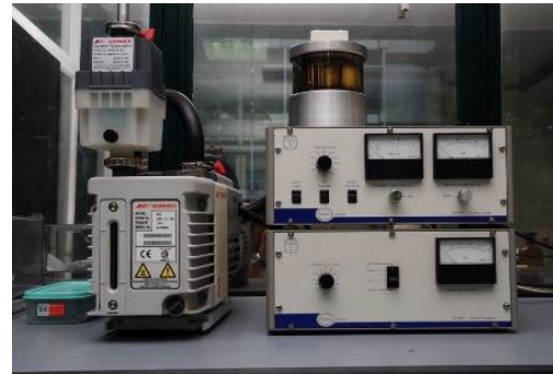
Equipment for deposition of thin films and electrodes (a) VUP-5; (b) SC7620 and CA7625
