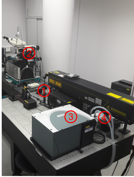
Figure 2.4: Picture of the \mu PL setup used. (1) laser diode used for excitation, (2) confocal microscope, (3) spectrometer, (4) camera.
